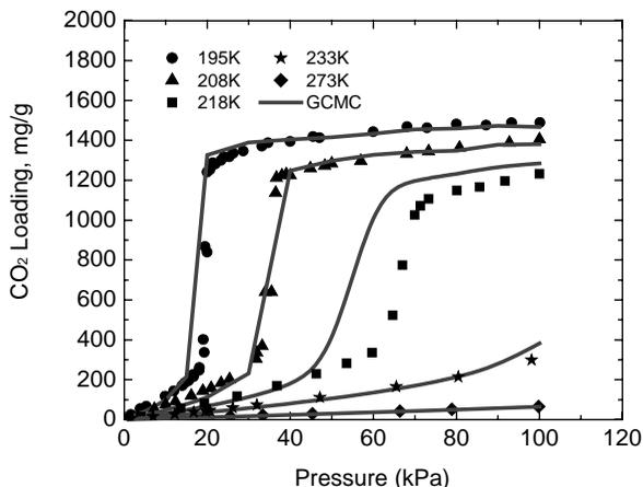
**FIGURE 11.4** Comparison of GCMC simulations and experimental adsorption isotherms for  $\text{CO}_2$  in IRMOF-1. (Reprinted with permission from ref. 51. Copyright © 2008 American Chemical Society).
