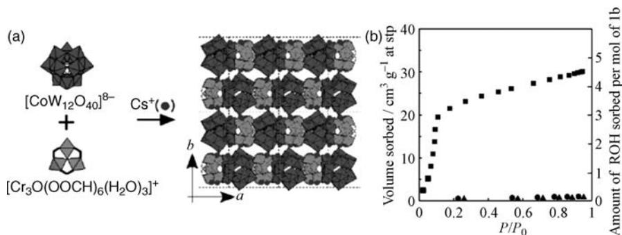
**FIGURE 7.23** (a) Synthesis and crystal structure ( $ab$  plane) of  $\text{Cs}_5[\text{Cr}_3\text{O}(\text{OOCH})_6(\text{H}_2\text{O})_3][\alpha\text{-CoW}_{12}\text{O}_{40}]\cdot 7.5\text{H}_2\text{O}$ , water (■,  $P_0 = 3.06$  kPa), methanol (●,  $P_0 = 15.6$  kPa), and ethanol (▲,  $P_0 = 6.67$  kPa) sorption isotherms of the evacuated material at 298 K.
