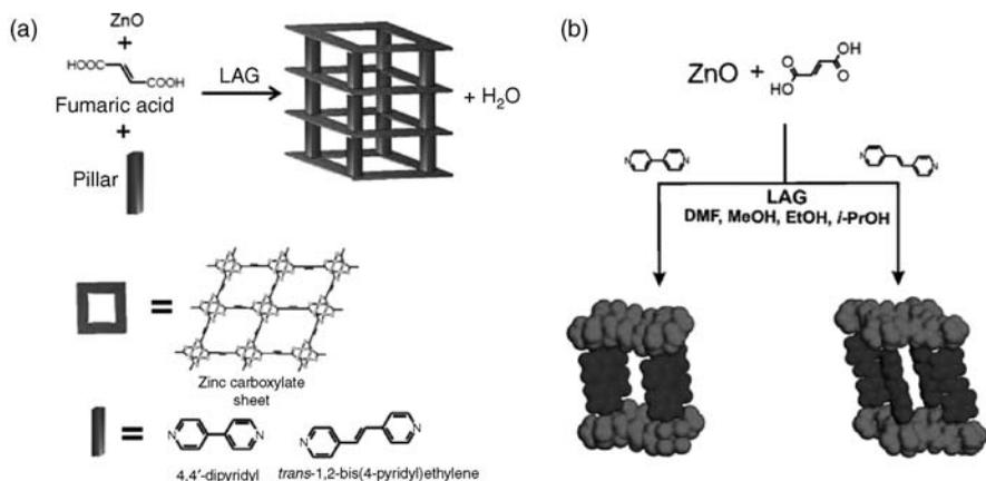
**FIGURE 9.24** (a and b) Synthesis of pillared open MOFs from zinc oxide and fumaric acid by using LAG.<sup>23</sup>
