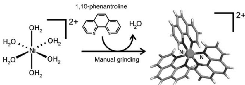
**FIGURE 9.5** Mechanochemical replacement of water ligands on an octahedral  $\text{Ni}^{2+}$  ion with 1,10-phenanthroline.<sup>62</sup> The counter ion is nitrate.
