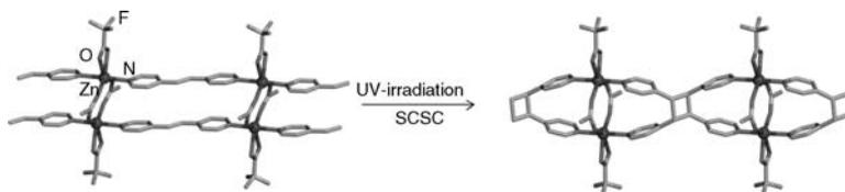
**FIGURE 10.2** Representation of SCSC [2 + 2] cycloaddition reaction of  $[\{\text{CF}_3\text{CO}_2\}(\mu\text{-O}_2\text{CCH}_3)\text{Zn}]_2(\mu\text{-bpe})_2$ . Hydrogen atoms omitted for clarity.
