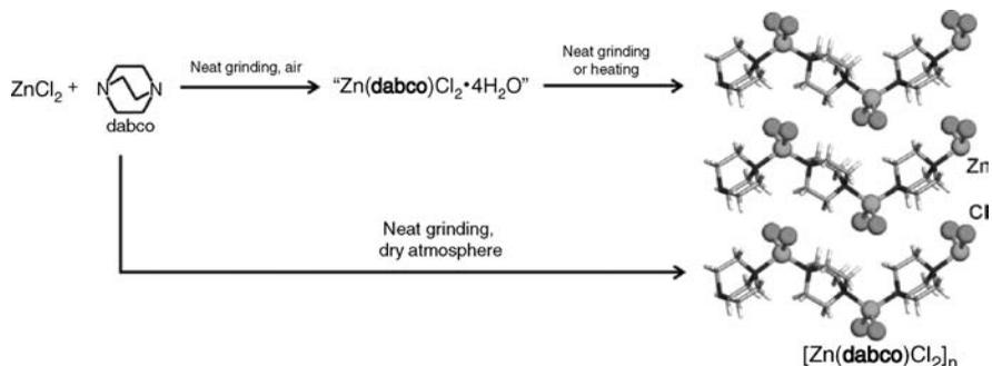
**FIGURE 9.11** The formation of the  $[\text{Zn}(\text{dabco})\text{Cl}_2]_n$  coordination polymer by manual grinding in air and grinding in a dry atmosphere.<sup>64</sup>
