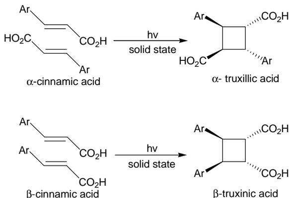
**SCHEME 10.1** Schematic view of solid-state reactions of two polymorphic forms of cinnamic acid.
