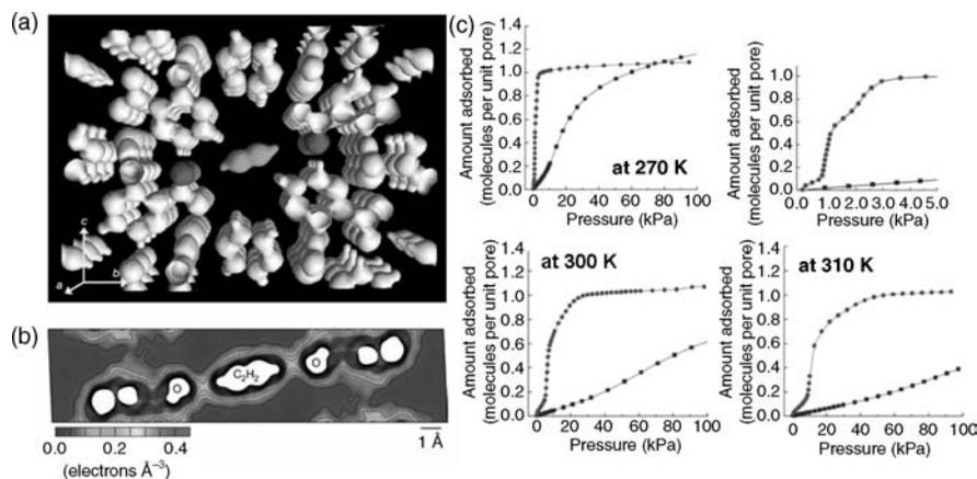
**FIGURE 7.15** (a) MEM electron densities of  $\text{C}_2\text{H}_2$  adsorbed  $[\text{Cu}_2(\text{pzdc})_2(\text{pyz})]$  at 170 K, (b) MEM electron density distribution views on the 2D section defined by the molecular axis of the  $\text{C}_2\text{H}_2$  molecule, and (c) adsorption isotherms for  $\text{C}_2\text{H}_2$  (circles) and  $\text{CO}_2$  (squares) on  $[\text{Cu}_2(\text{pzdc})_2(\text{pyz})]$ . (The inset shows the lower  $P/P_0$  region at 270 K.)
