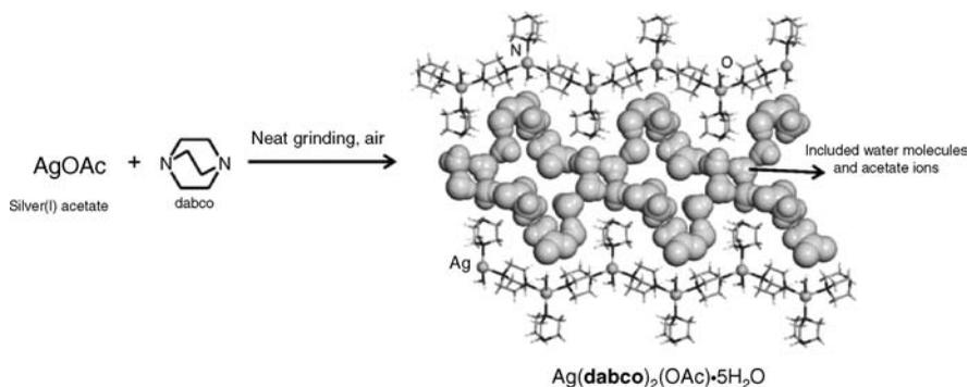
**FIGURE 9.13** Formation of a hydrated coordination polymer by neat manual grinding of silver(I) acetate and **dabco** in air. The water molecules and acetate ions that act as guests in the lattice host self-assembled from cationic chains  $[\text{Ag}(\text{dabco})_2(\text{H}_2\text{O})]_n^{n+}$  are shown using the space-filling model.<sup>64</sup>
