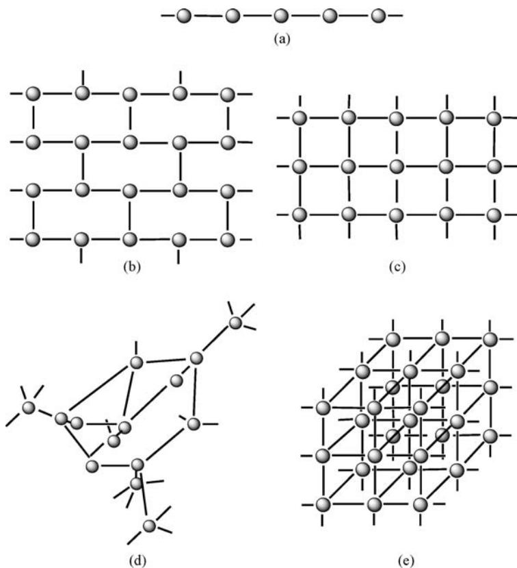
**SCHEME 4.1** The modular, building block approach to the synthesis of metal-organic frameworks has been successfully demonstrated by the synthesis of a range of framework materials with (a) 2-connected, (b) 3-connected, (c) 4-connected square-planar, (d) 4-connected tetrahedral, and (e) 6-connected metal-organic frameworks.
