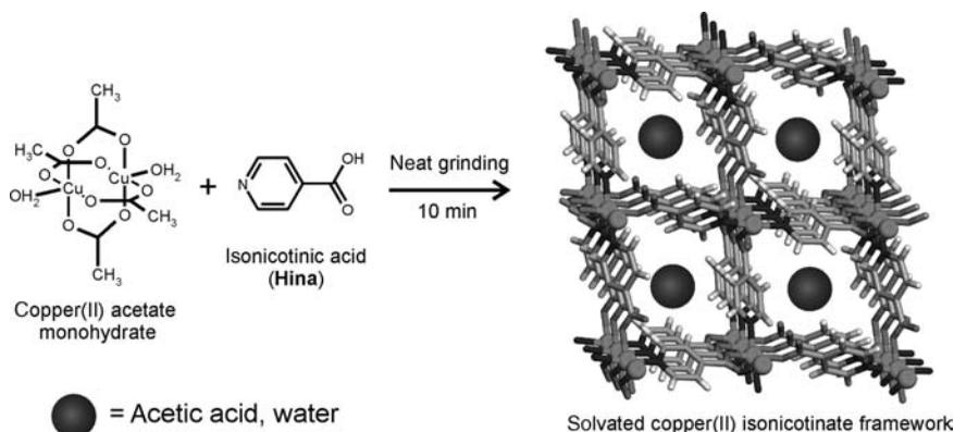
**FIGURE 9.16** Mechanochemical synthesis of a porous MOF by neat grinding.<sup>22</sup>
