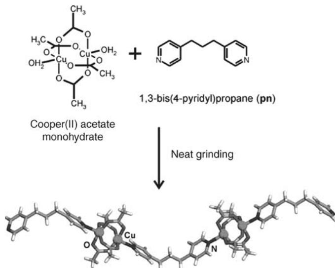
**FIGURE 9.9** Mechanochemical construction of a 1D coordination polymer.<sup>21</sup>
