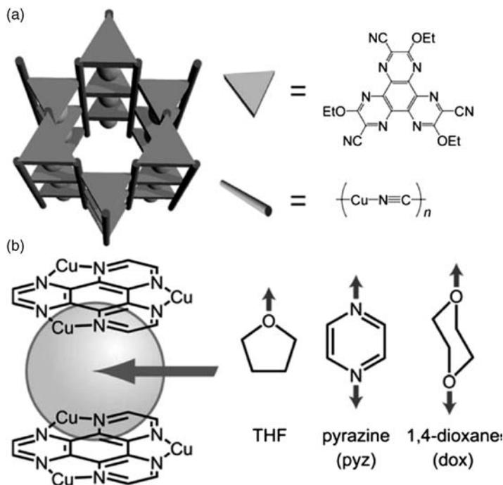
**FIGURE 5.12** Schematic representation of the (a) framework  $\{[\text{Cu}^{\text{I}}_3(\text{CN})_3\{\text{hat}(\text{CN})_3(\text{OEt})_3\}]\cdot 3\text{THF}\}_n$  and (b) inclusion of solvent guest molecules into pores comprising  $\pi$  planes.
