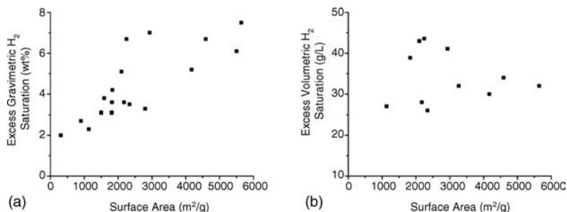
**FIGURE 8.5** Correlation between surface area and (a) excess gravimetric saturation at 77 K, (b) excess volumetric hydrogen saturation at 77 K.
