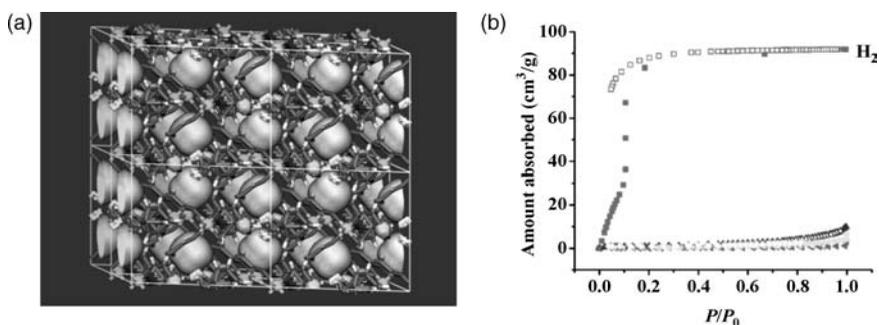
**FIGURE 7.4** (a) The Connolly surface of  $[Cu_2(fum)_2(bpe)]$  with the inner walls of pocket-like pores. (b) The gas sorption isotherms for  $H_2$  (squares) over  $N_2$  (triangles), Ar (inverted triangles), and CO (diamonds) at 77K. Solid symbol = adsorption, open symbol = desorption.
