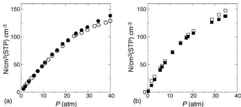
**FIGURE 11.3** Experimental and simulated methane adsorption isotherms at 298 K in (a) IRMOF-1 and (b) IRMOF-6 (open symbols, experimental results; closed symbols, simulation results). (Reprinted with permission from ref. 39. Copyright © 2004 American Chemical Society).
