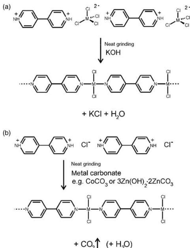
**FIGURE 9.7** Two applications of neutralization in assisting the mechanochemistry of coordination polymers: (a) by the addition of an external reagent (KOH) and (b) by using a metal salt of a basic anion, such as carbonate or hydroxide.
