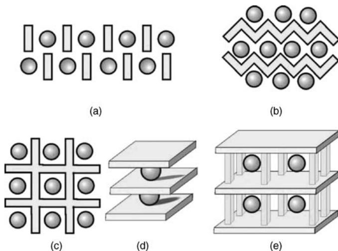
**FIGURE 9.1** Types of inclusion compounds involving discrete (A), one-dimensional (B), two-dimensional (C and D), and three-dimensional (E) metal–organic hosts. The host structure is shown in black, while the gray circles represent guest molecules.
