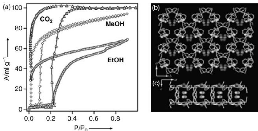
**FIGURE 7.22** (a) Sorption isotherms of CO<sub>2</sub> (195 K), MeOH, and EtOH (298 K) for [Cu(pyrdc)(bpp)]. Honeycomb-like 2D layer with CO<sub>2</sub> molecules along the *c*-axis (b) and *b*-axis (c).
