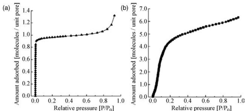
**FIGURE 7.25** (a) Adsorption isotherm for benzene of CPL-2 at 300 K in the relative pressure range from  $10^{-4}$  to 0.95 ( $P_0 = 14.6$  kPa). (b) Adsorption isotherm for water of CPL-2 at 300 K in the relative pressure range from  $10^{-3}$  to 1.0 ( $P_0 = 3.53$  kPa).
