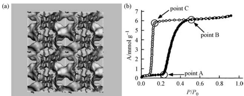
**FIGURE 7.21** (a) The Connolly surface of [ $\text{Cu}_2(\text{pzdc})_2(\text{dpyg})$ ] with the pore walls. (b) Methanol adsorption (filled circles) and desorption (open circles) isotherms of [ $\text{Cu}_2(\text{pzdc})_2(\text{dpyg})$ ] at 298 K (point A – a sudden rise, point B – a saturated level, and point C – an abrupt drop).
