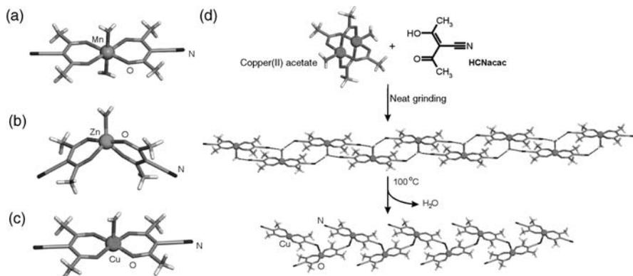
**FIGURE 9.19** Molecular structures of: (a)  $\text{Mn}(\text{CNacac})_2(\text{H}_2\text{O})_2$ ; (b)  $\text{Zn}(\text{CNacac})_2(\text{H}_2\text{O})$ ; (c)  $\text{Cu}(\text{CNacac})_2(\text{H}_2\text{O})$  and (d) construction of the  $\text{Cu}(\text{CNacac})_2$  coordination polymer by a neat grinding-annealing sequence, starting from copper(II) acetate and  $\text{HCNacac}$ .<sup>48</sup>
