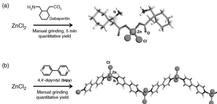
**FIGURE 9.4** Manual grinding synthesis of: (a) a metal–organic derivative of the drug gabapentin<sup>61</sup> and (b) the orthorhombic polymorph of the  $[\text{ZnCl}_2(\text{bipy})]_n$  polymer.<sup>50</sup>
