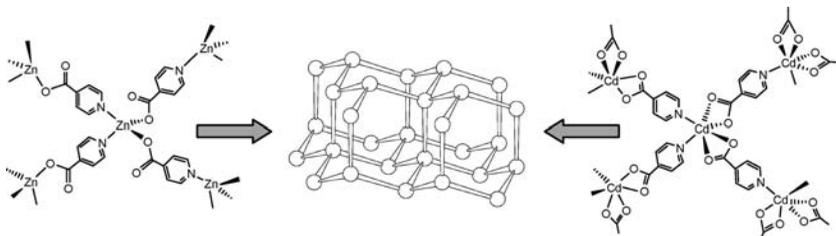
**SCHEME 6.1** Linking of *p*-pyridinecarboxylate ligands by Zn<sup>2+</sup> and Cd<sup>2+</sup> ions to lead to 3D MOFs with the diamondoid topology.
