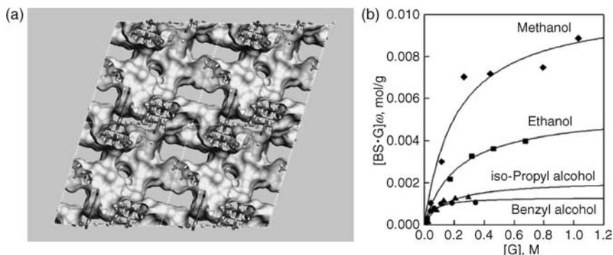
**FIGURE 7.30** (a) The Connolly surface of **BOF-1** with the pore walls. (b) A plot of the amount of sorption by dried solid **BOF-1** (powder form) with different alcohols in toluene with respect to their concentration.
