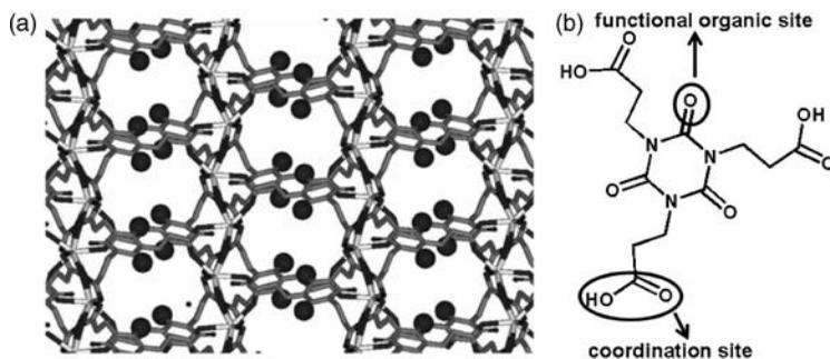
**FIGURE 5.7** (a) View of the 3D structure of  $\{[\text{Ln}(\text{tci})\cdot\text{H}_2\text{O}]\cdot 4\text{H}_2\text{O}\}_n$ . Basic functional groups in the pore surface are highlighted. (b) Functional site and coordination sites are marked in the ligand.
