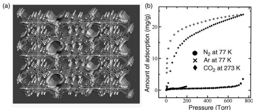
**FIGURE 7.1** (a) The Connolly surface of  $[\text{Er}_2(\text{pda})_3]$  with the pore walls. (b) Gas sorption isotherms for  $\text{N}_2$ , Ar (77 K), and  $\text{CO}_2$  (273 K).
