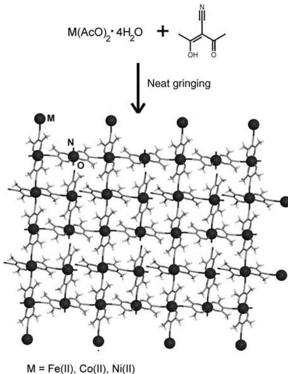
**FIGURE 9.17** Neat grinding synthesis of the non-porous 3D MOFs by grinding.<sup>48</sup>
