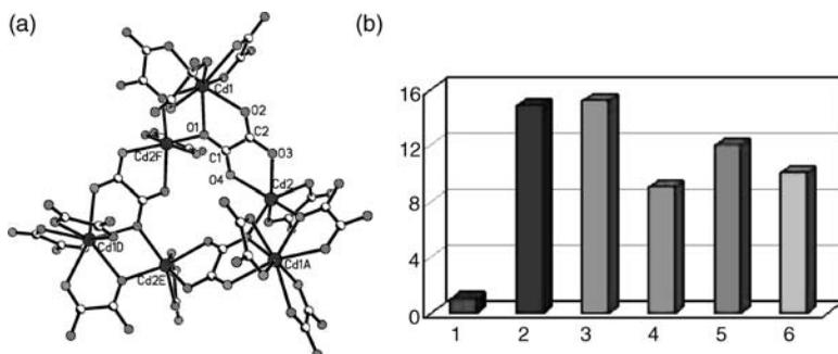
**FIGURE 6.15** (a) A view of the octupolar 3D anionic open framework of **19**. (b) A comparison of the SHG intensities of KDP, **19**, the  $\text{NH}_4^+$ ,  $\text{Na}^+$ ,  $\text{K}^+$  exchanged samples of **19**, and **18** (from left to right; the intensity of KDP is set as 1).
