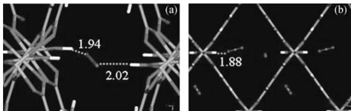
**FIGURE 11.7** (a) The double interaction of a  $\text{CO}_2$  molecule with the MIL-53np (Al) structure and (b) the interaction of a  $\text{CO}_2$  molecule with a single  $\mu_2\text{-OH}$  group in MIL-53lp (Al).<sup>56</sup> (Reproduced by permission from the Royal Society of Chemistry).
