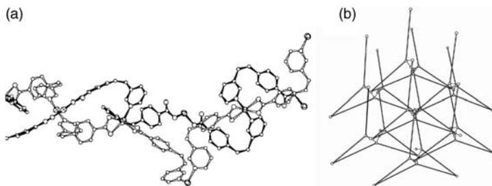
**FIGURE 6.18** (a) A view of the cross-link between a primary and a secondary helix in **28**. (b) A perspective view of **28** slightly away from the  $c$  axis showing the 3D network resulting from the crosslinking of primary and secondary helices. Only Zn atoms are shown.
