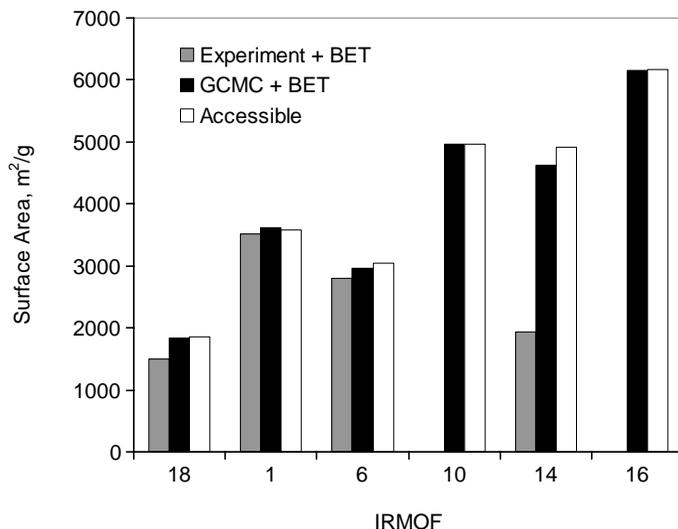
**FIGURE 11.8** Comparison of IRMOF surface areas obtained from the BET theory applied to experimental N<sub>2</sub> isotherms, surface areas from the BET theory applied to simulated N<sub>2</sub> isotherms, and accessible surface areas calculated from the crystal structures. (Reprinted with permission from ref. 41. Copyright © 2007 American Chemical Society).
