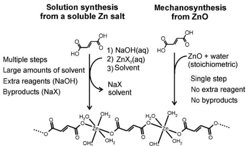
**FIGURE 9.8** Comparison of solution-based synthesis of a coordination polymer to the mechanochemical synthesis starting from the metal oxide.
