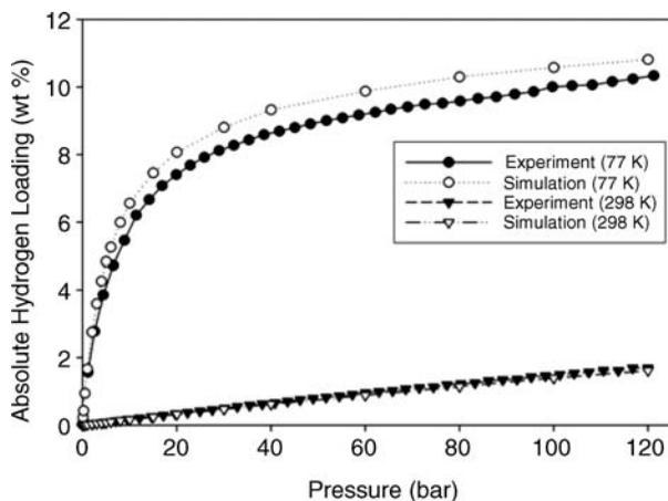
**FIGURE 11.11** Hydrogen adsorption isotherms (absolute quantities) in IRMOF-1 at 77 and 298 K. GCMC simulations<sup>91</sup> agree well with experimental measurements of Kaye et al.<sup>92</sup>
