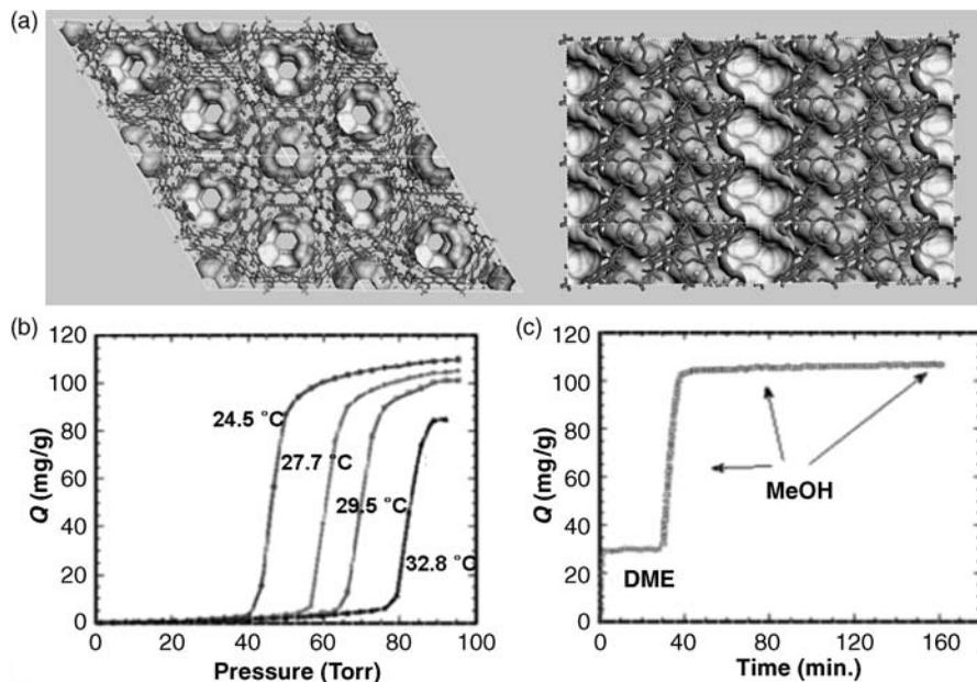
**FIGURE 7.26** (a) The Connolly surface of [Zn(tbip)] with the pore walls along the  $c$ -axis. (b) MeOH adsorption isotherms at different temperatures. (c) Adsorption of DME at 30 °C followed by MeOH on [Zn(tbip)].
