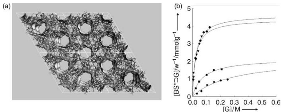
**FIGURE 7.31** (a) The Connolly surface of  $[\text{Ni}(\text{cyclam})(\text{bpydc})]$  with the pore walls. (b) Binding of host solid  $[\text{Ni}(\text{cyclam})(\text{bpydc})]$  with the organic guests EtOH (●), PhOH (▼), pyridine (■), and benzene (◆).  $K_f$ ,  $[G]$ , and  $[\text{BS} \supset G]/w$  are defined as binding constant, concentration of guest (G), and binding sites of the host to the guest (G), respectively.
