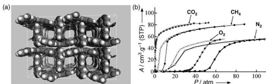
**FIGURE 7.18** (a) The Connolly surface of  $[Cu(dhbz)_2(bpy)]$  with the pore walls. (b) Adsorption (filled circles) and desorption (open circles) isotherms of  $N_2$ ,  $CH_4$ ,  $CO_2$ , and  $O_2$  at 298 K.
