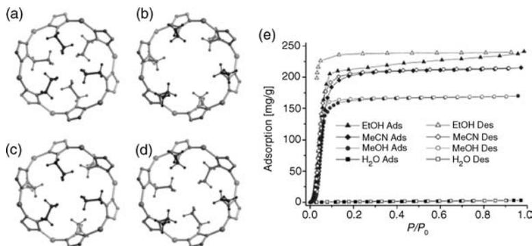
**FIGURE 5.11** (a–d) Perspective view of the four different states of the pore containing hydrophobic ethyl groups derived from the crystal structure of  $[\text{Cu}(\text{etz})]_{\infty}$ , and (e)  $\text{H}_2\text{O}$ , MeOH, EtOH, and MeCN sorption isotherms.
