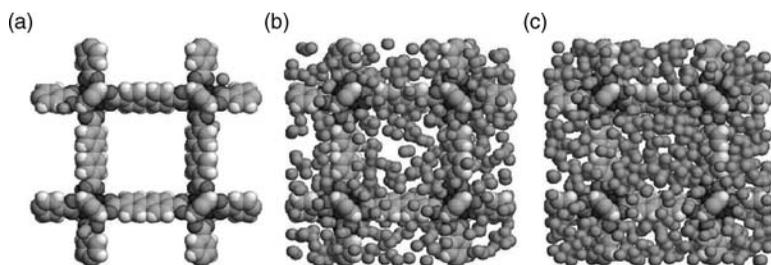
**FIGURE 11.13** Snapshots of hydrogen adsorption in IRMOF-10 at 77 K from GCMC simulation at (a) 0.1 bar, (b) 30 bar, and (c) 120 bar. (Reprinted with permission from ref. 91. Copyright © 2006 American Chemical Society).
