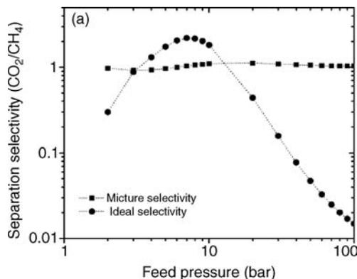
**FIGURE 7.35** Predicted ideal (circles) and mixture (squares) permeation selectivities for a 10- $\mu\text{m}$ -thick MOF-5 membrane with a transmembrane pressure drop of 1.38 bar. Mixture selectivities are based on an equimolar feed.
