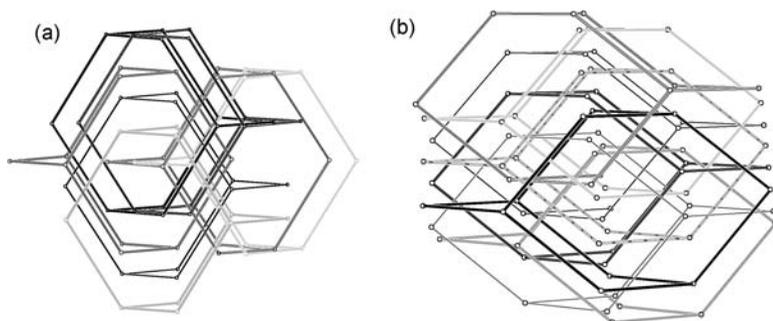
**FIGURE 6.4** (a) Diagram showing the sevenfold interpenetration in **6**. (b) Diagram showing the eightfold interpenetration in **7** and **8**.
