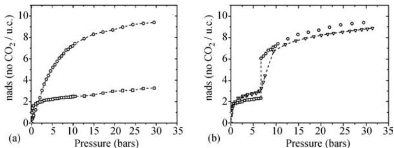
**FIGURE 11.6** (a) Simulated absolute adsorption isotherms for CO<sub>2</sub> in two different forms of MIL-53, MIL-53np (Al) (squares) and MIL-53lp (Al) (circles). (b) The simulations (circles) are compared with the experimental data (triangles).<sup>56</sup> (Reproduced by permission from the Royal Society of Chemistry).
