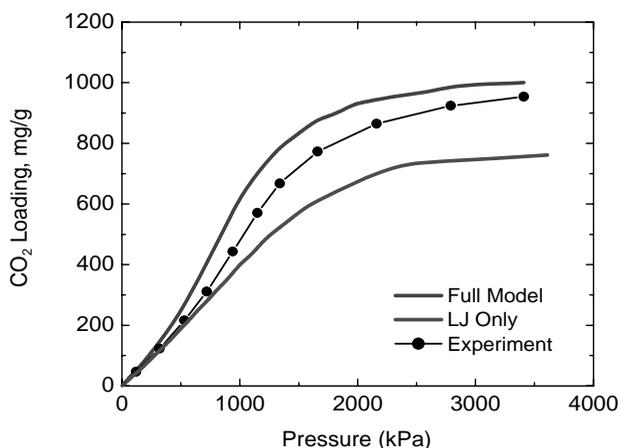
**FIGURE 11.5** Comparison of GCMC simulations and experimental adsorption isotherms for  $\text{CO}_2$  in IRMOF-1 at 298 K. The top curve was calculated from a model that included electrostatic effects. The bottom curve was calculated considering only the Lennard–Jones interactions. (Reprinted with permission from ref. 51. Copyright © 2008 American Chemical Society).
