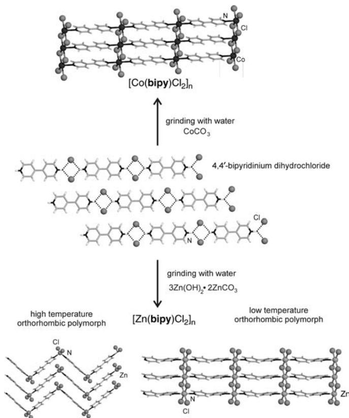
**FIGURE 9.22** Mechanochemical synthesis of coordination polymers using a transition metal carbonate or a basic carbonate as starting materials.<sup>51</sup>
