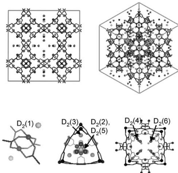
**FIGURE 8.3**  $D_2$  sites in HKUST-1, identified via neutron powder diffraction, numbered in order of occupation with increased loading. Top: shown along [001] (left) and [111] (right). Bottom: axial Cu(II) paddlewheel UMC site (left), along [111] in the 5 Å small pore with 3.5 Å side windows (middle), and along [100] showing the 9 Å pore. Reprinted with permission from Reference 46. Copyright 2006, American Chemical Society.
