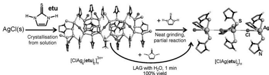
**FIGURE 9.3** Mechanochemical transformation of the [ClAg<sub>4</sub>(ethylenethiourea)<sub>6</sub>]<sup>3+</sup> coordination polymer into AgCl(ethylenethiourea)<sub>3</sub>, accelerated by small quantities of water.<sup>47</sup>
