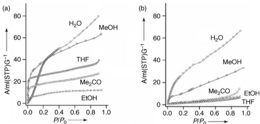
**FIGURE 7.20** Vapor sorption of [Cd(pzdc)(azpy)] (a) and [Cd(pzdc)(bpee)] (b) at 298 K,  $P_0$  is the saturated vapor pressure at 298 K; 3.17 kPa ( $\text{H}_2\text{O}$ ), 16.94 kPa (MeOH), 7.87 kPa (EtOH), 23.45 kPa (THF), and 30.59 kPa ( $\text{Me}_2\text{CO}$ ).
