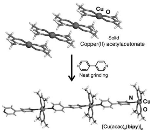
**FIGURE 9.10** Mechanochemical construction of a 1D coordination polymer from copper(II) acetylacetonate and **bipy**, reported by Pichon and James.<sup>52</sup>
