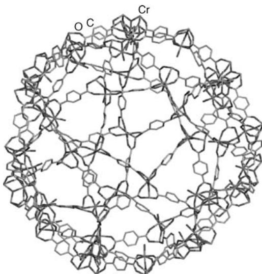
**FIGURE 9.26** Fragment of the giant pore MOF MIL-101, constructed by microwave-assisted synthesis.<sup>15</sup>
