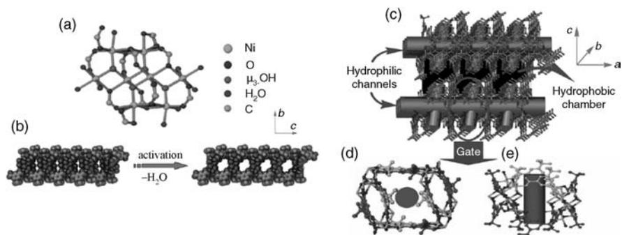
**FIGURE 7.9** Crystal structure of  $[\text{Ni}_8(\text{tbip})_6(\mu_3\text{-OH})_4(\text{OH}_2)_8]\cdot 8\text{H}_2\text{O}$ . (a) Structure of the octanickel cluster. (b) Structures of solvated and desolvated trilayers. The desolvated trilayer displays hydrophilic channels along the  $a$ -axis. (c) Two trilayers pack along the  $c$ -axis to form hydrophobic chambers. Top and side views of  $\text{tbip}$  pairs.
