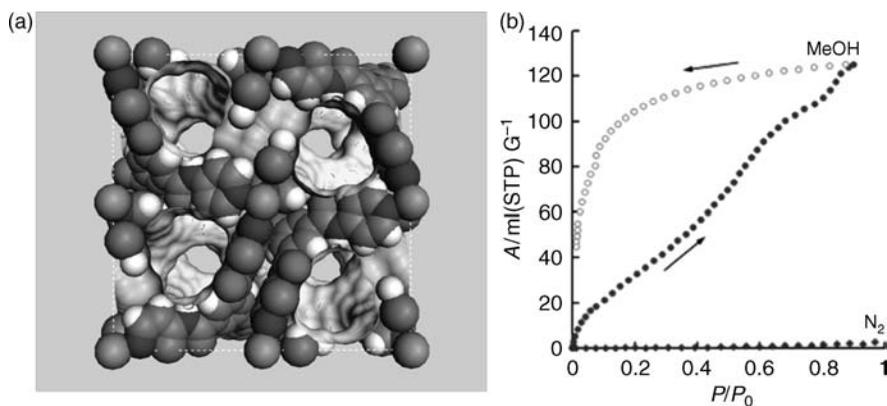
**FIGURE 7.19** (a) The Connolly surface of [Cd(4-btapa)<sub>2</sub>(NO<sub>3</sub>)<sub>2</sub>] with the pore walls. (b) Gas adsorption–desorption isotherms of [Cd(4-btapa)<sub>2</sub>(NO<sub>3</sub>)<sub>2</sub>] for N<sub>2</sub> and MeOH.  $P_0$  is the saturated vapor pressure, 101.3 kPa, of N<sub>2</sub> (77 K), and 16.94 kPa, of methanol (298 K).
