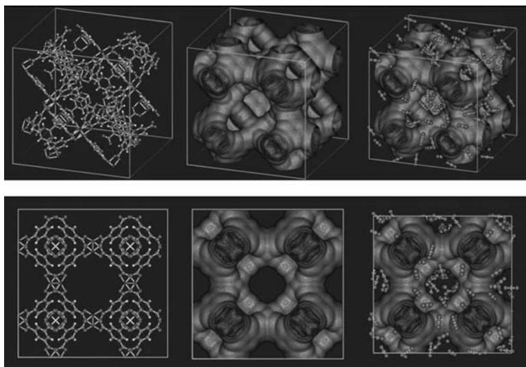
**FIGURE 11.2** The Cu-BTC metal–organic framework: (left) ball and stick, (middle) the adsorption surface, and (right) snapshot of CO<sub>2</sub> at 298 K close to maximum loading.
