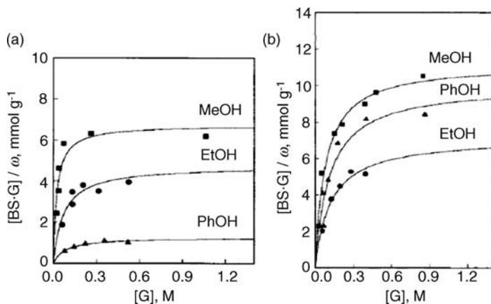
**FIGURE 7.33** The sorption uptakes of MeOH, EtOH, and PhOH by  $[\text{Ni}(\text{C}_{20}\text{H}_{32}\text{N}_8)] [\text{C}_6\text{H}_9(\text{COOH})_2(\text{COO})]_2$  (a) and  $[\text{Ni}(\text{C}_{20}\text{H}_{32}\text{N}_8)]_3[\text{C}_6\text{H}_9(\text{COO})_3]_2$  (b).
