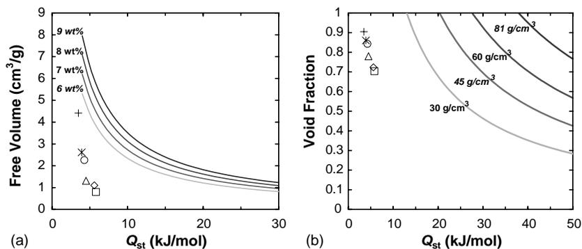
**FIGURE 11.14** (a) Requirements for target gravimetric loadings at 120 bar and 298 K. (b) Requirements for target volumetric loadings at 120 bar and 298 K.  $\triangle$ , IRMOF-1;  $\diamond$ , IRMOF-9; \*, IRMOF-10;  $\circ$ , IRMOF-14; +, IRMOF-16;  $\square$ , Cu-BTC. (Reprinted with permission from ref. 93. Copyright © 2007 American Chemical Society).
