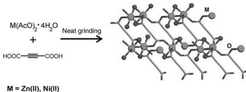
**FIGURE 9.18** Mechanochemical synthesis of a 3D non-porous polymer by neat grinding of zinc(II) or nickel(II) acetate tetrahydrate with **Hadc**. The metal(II) ions and oxygen atoms of water molecules are shown as black and dark gray spheres, respectively, whereas the oxygen (light gray) and carbon (gray) atoms of **adc**<sup>−</sup> ligands are displayed using the wireframe model.<sup>52</sup>
