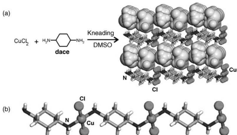
**FIGURE 9.23** (a) The construction of a metal–organic clay mimic material by kneading copper(II) chloride and dace in the presence of DMSO (or water) and (b) a single chain of  $[\text{Cu}(\text{dace})\text{Cl}_2]_n$ . Solvent molecules included between the layers of  $[\text{Cu}(\text{dace})\text{Cl}_2]_n$  are shown using the space-filling model.<sup>56</sup>
