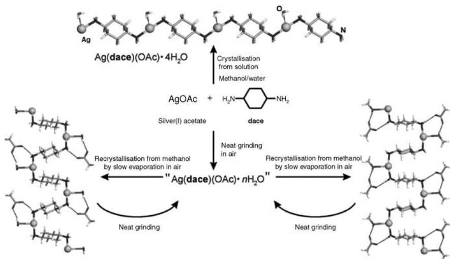
**FIGURE 9.14** Construction of solvated coordination polymers from silver(I) acetate and **dace** by mechanochemical and solution routes.<sup>53</sup>
