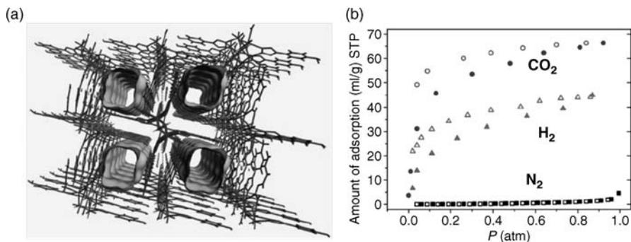
**FIGURE 7.14** (a) The top view of  $[\text{Cd}_3(\text{aptz})(\mu_3\text{-OH})_2(\text{OH}_2)_2]$  with  $2 \times 2$  arrays of the 1D channels. (b) Gas sorption isotherms of  $\text{N}_2$  (77 K),  $\text{H}_2$  (77 K), and  $\text{CO}_2$  (195 K) (solid symbol = adsorption, open symbol = desorption).
