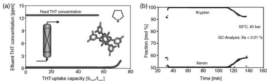
**FIGURE 7.34** (a) Breakthrough curve of continuous tetrahydrothiophene removal from nature gas using  $[\text{Cu}_3(\text{BTC})_2(\text{H}_2\text{O})_3]$  out of electrochemical synthesis. (b) Separation of Kr-Xe gas mixture by continuous adsorption on electrochemically produced  $[\text{Cu}_3(\text{BTC})_2(\text{H}_2\text{O})_3]$ .
