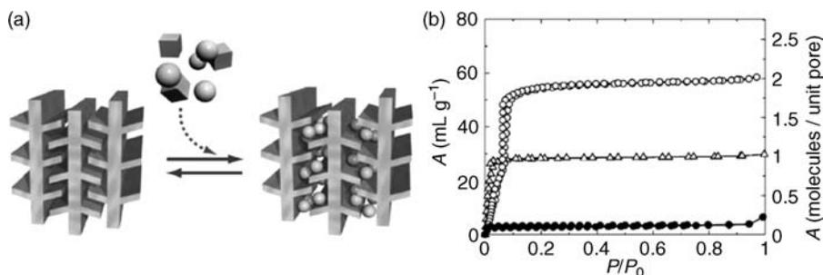
**FIGURE 7.24** (a) Representation of selective guest sorption of a coordination polymer with interdigitated structure. (b) Adsorption and desorption isotherms of methanol (open circles), ethanol (open triangles), and benzene (closed circles) for activated CID-1 at 298 K.
