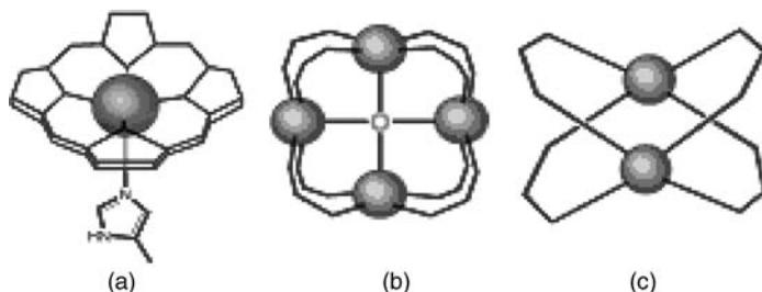
**FIGURE 8.2** (a) Schematic drawing of the active center of hemoglobin; the gold sphere represents an iron atom. (b) Schematic drawing of the tetranuclear  $M_4(\mu_4-O)(CO_2)_8$  SBU containing coordinatively unsaturated metal atoms. (c) The  $M_2(CO_2)_4$  paddlewheel SBU.
