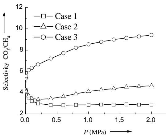
**FIGURE 11.9** Effect of electrostatic interactions on the selectivity of CO<sub>2</sub> from equimolar mixtures of methane and CO<sub>2</sub> in Cu-BTC at 298 K. (From ref. 65. Copyright © Wiley-VCH. Reproduced with permission).
