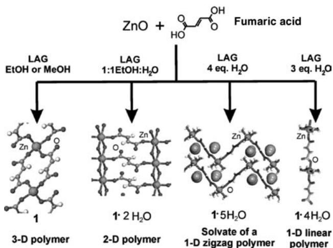
FIGURE 9.21 Screening for coordination polymers from **ZnO**, using LAG.<sup>23</sup>
