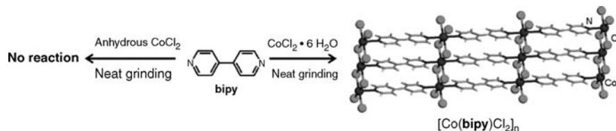
**FIGURE 9.12** Mechanochemical reactivity of **bipy** towards anhydrous  $\text{CoCl}_2$  and  $\text{CoCl}_2 \cdot 6\text{H}_2\text{O}$ .<sup>50</sup>
