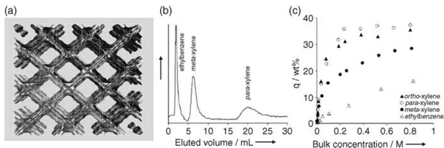
**FIGURE 7.28** (a) The Connolly surface of [V<sup>III</sup>(OH)(bdc)] with pore walls along the *a*-axis. (b) Chromatographic separation of a mixture of ethylbenzene, *meta*- and *para*-xylene on a column packed with MIL-47 in the liquid phase, with hexane as the desorbent at 298 K. The signal intensity of the refractive index detector is shown versus the eluted volume. (c) Adsorption isotherms of guest molecules on MIL-47 at 298 K.
