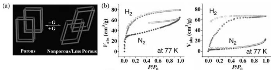
**FIGURE 7.5** (a) Schematic illustration of the structural transformation. (b) Gas sorption isotherms for  $[\text{Co}_2(\text{ndc})_2(\text{bpy})]$  after activation at 150 °C (left) and 200 °C (right).
