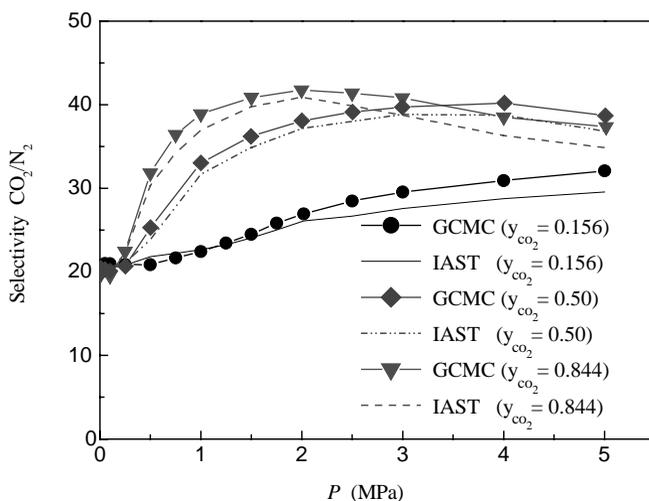
**FIGURE 11.10** Selectivities for CO<sub>2</sub> from binary mixtures of CO<sub>2</sub> and N<sub>2</sub> with three gas compositions in Cu-BTC at 298 K. Results from binary GCMC simulations are compared with results using simulated single-component isotherms and ideal adsorbed solution theory. (From ref. 64. Copyright © 2007 John Wiley & Sons, Inc. Reprinted with permission).
