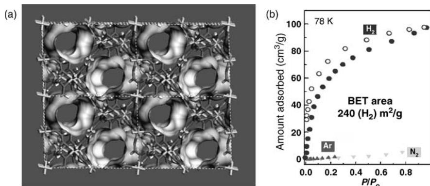
**FIGURE 7.2** (a) The Connolly surface of  $[\text{Mn}(\text{HCOO})_2]$  with the pore walls. (b) Gas sorption isotherms of  $\text{N}_2$ , Ar, and  $\text{H}_2$  at 78 K for  $[\text{Mn}(\text{HCOO})_2]$ .
